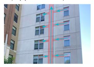
In another building, a lounge was proposed to be converted to a testing space. Strategies included directed pedestrian traffic flow, isolation of the space by means of a dedicated ventilation system ensuring negative pressure and exhausting air directly to the exterior, introducing a hand sink and accessories, and temporary toilet facilities adjacent to the suite outside the building. See below floor plan.
